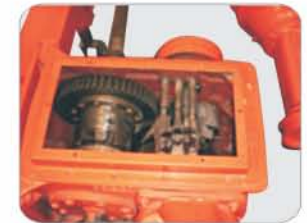
Heavy duty gearbox with five speeds Collar shift gears
