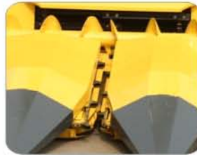
Stalk Rollers Fitted with Blades of Sharp & Hardened Edge For Long Service.
