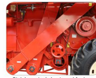
Stainless steel sheet used for long life of parts which are subjected to more wearing like elevators Used UCF bearing is widely appreciated for durability and long serviceability
