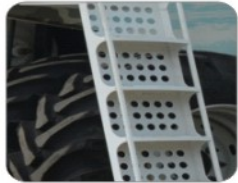
Ladder cover with sheet for safety purpose
