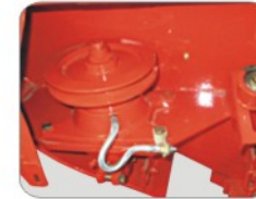
Cutting blade driven thru. Gear mechanism
