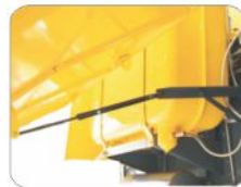
Gas spring used for opening of shields.
