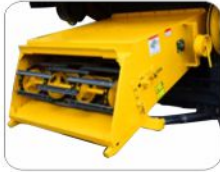
Feeder chamber length increased. Single sheet bending
