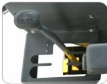
Single lever for shift gears
