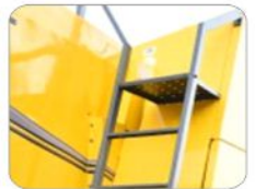
Resting platform on rear ladder.
