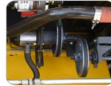
High capacity hydraulic pump used (26L).
