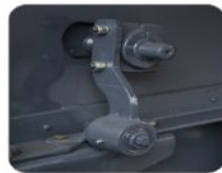
Heavy duty sieve box bracket
