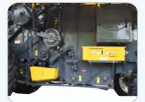
Single sheet used for Chassis design. Wide windows in chassis for easy maintenance
