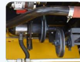
High capacity hydraulic pump used (26L).
