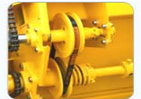
Variator pulley used for rpm adjustment of reel.
