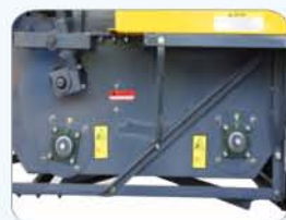
EN-42 sheet used for long life of auger casing
