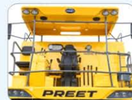
Newly design heavy duty front railing
