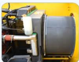
Better quality brush used for Radiator cleaning with belts operated brush.
