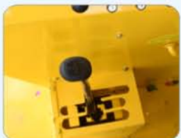
Single lever for shift gears
