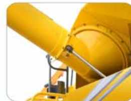
Hydraulically operated discharge tube for quick engage and disengagement without any extra labour. Less maintenance
