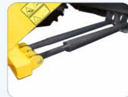
Heavy duty hydraulic cylinder Used (75mm.)
