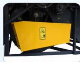
Blower dia increased for better cleaning Newly designed blower covers
