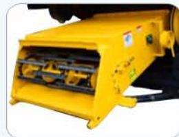
Feeder chamber length increased. Single sheet bending
