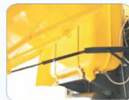
Gas spring used for opening of shields.
