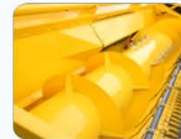
Front auger of 16" dia.
