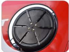
Engine cooling by clean air through rotating sieve equipped with additional fan
