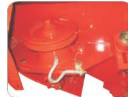
Cutting blade driven thru. Gear mechanism
