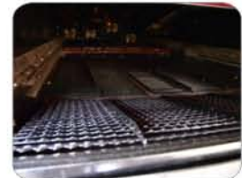
Large sieve area for optimum grain cleaning
