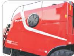
Bigger shields covering rotated parts with extra safety
