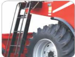
Ladder cover with sheet for safety purpose
