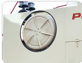
Engine cooling by clean air through rotating sieve
