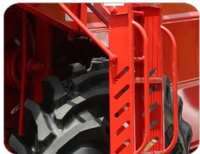
Ladder cover with sheet for safety purpose
