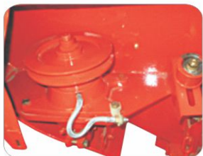
Cutting blade driven thru. Gear mechanism
