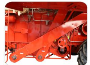
Stainless steel sheet used for long life of parts which are subjected to more wearing like elevators. Used UCF bearing is widely appreciated for durability and long serviceability
