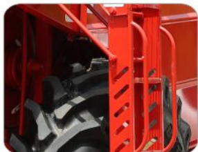
Ladder cover with sheet for safety purpose
