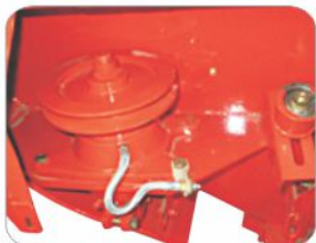
Cutting blade driven thru. Gear mechanism
