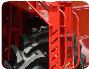
Ladder cover with sheet for safety purpose
