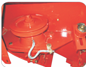
Cutting blade driven thru. Gear mechanism
