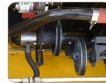
High capacity hydraulic pump used (26L).
