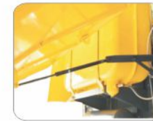
Gas spring used for opening of shields.
