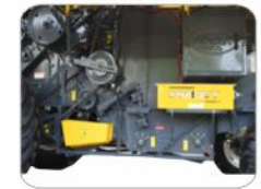
Single sheet used for Chassis design. Wide windows in chassis for easy maintenance
