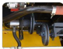
High capacity hydraulic pump used (26L).
