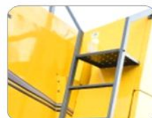
Resting platform on rear ladder.
