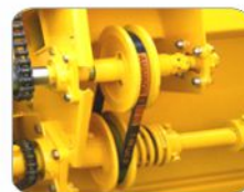
Variator pulley used for rpm adjustment of reel.
