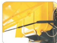
Gas spring used for opening of shields.
