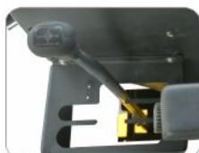
Single lever for shift gears
