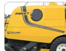
Newly designed shields covering rotating Parts with extra safety.
