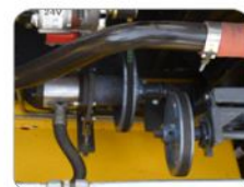
High capacity hydraulic pump used (26L).
