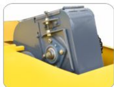
Elevator height increased for better Cleaning.
