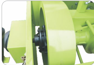
Heavy flywheel ensures smooth transmission and maximum Power transfer.
