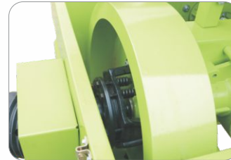
Slip clutch and shear bolt to secure the baler transmission.
