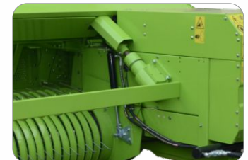
Hydraulic pick-up height adjustment
