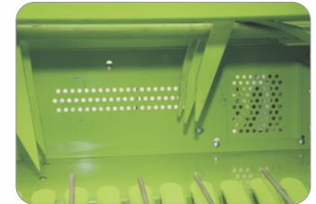
Each feeder tine is protected by a shear bolt.
