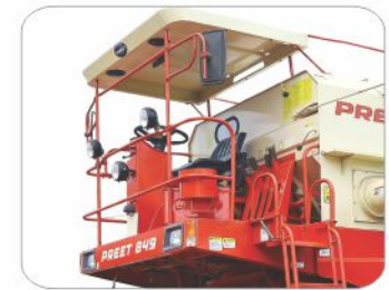
Broader Canopy Providing Extra Cover to the Operator Area Long Distance Focus Light Small Turning Radius
